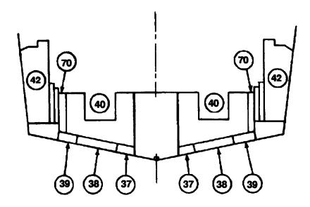
**BLOCK PLACEMENT DIAGRAM CROSS-SECTION (MK 1)**
