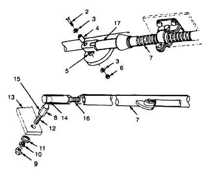
3. Remove bolt (2), two washers (3), spacer (4), spacer (5) and nut (6) using 9/16 inch wrench, socket and ratchet. This disconnects steering cable from tie rod (7).
