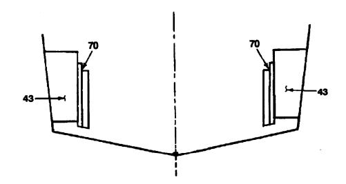
**BLOCK PLACEMENT CROSS-SECTION (MK 2)**
