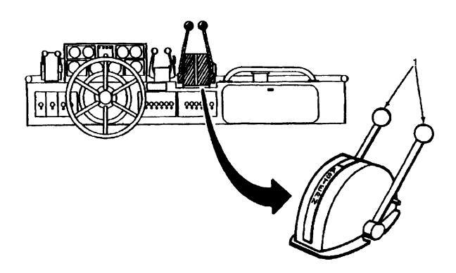
1. Move scoop control levers (1) to FULL FORWARD position.
