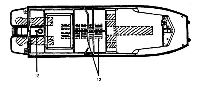
**1-9. LOCATION AND DESCRIPTION OF FORWARD COCKPIT AND CONTROL CONSOLE.** The console is located at the forward end of the boat and contains the controls necessary to operate the boat, the manual bilge pump, and stowage compartments.
