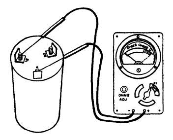
4. Check resistance between diode terminals by doing the five tests listed in the table below.
