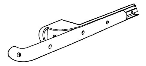
3. Remove section of fendering (rub rail) (5) from boat and lay out on flat surface.
