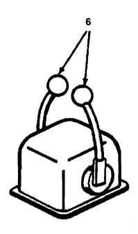
1. Rotate lever knob (6) counterclockwise.
