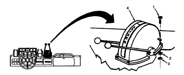
2. Using screwdriver and 10 mm open end wrench remove four screws (1), washers (2) and nuts (3) securing housing (4) to console and remove housing (4).
