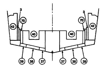
**BLOCK PLACEMENT DIAGRAM CROSS-SECTION (MK 1)**
