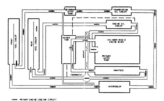
SECONDARY ENGINE COOLING CIRCUIT
