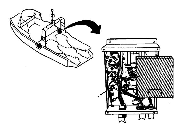
3. Using flat tip screwdriver remove two screws (1) from regulator box cover.
