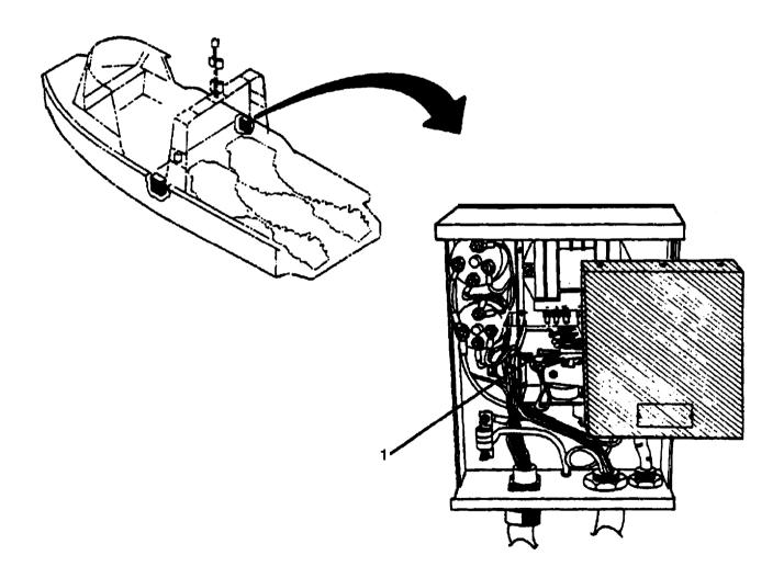
3. Using flat tip screwdriver remove two screws (1) from regulator box cover.
