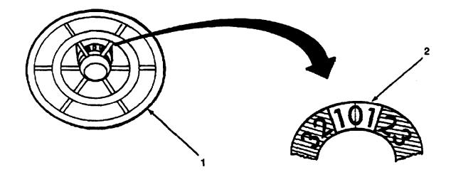
4. Turn steering wheel (1) until scoop position indicator (2) is on zero.
