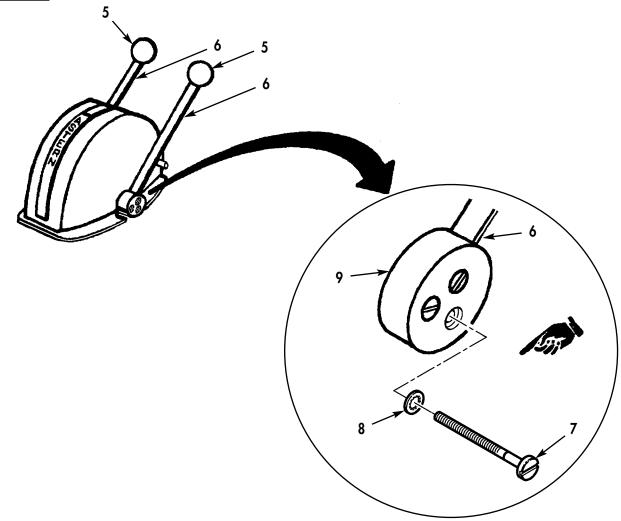
1. Using screwdriver reinstall three washers (8) and screws (7) securing lever (6) to hub (9).
