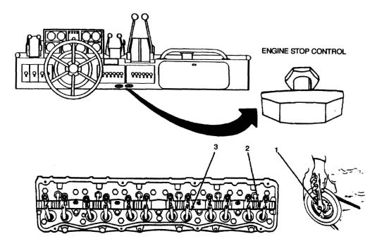
3. Using 15/16-inch open end wrench placed on nose bolt (1) of crankshaft pulley, turn engine counterclockwise until valves number 1 (2) and 4 (3) are opened by their respective rocker arms. Valves are open when rocker arm has pushed valve stem cap down as far as possible.
