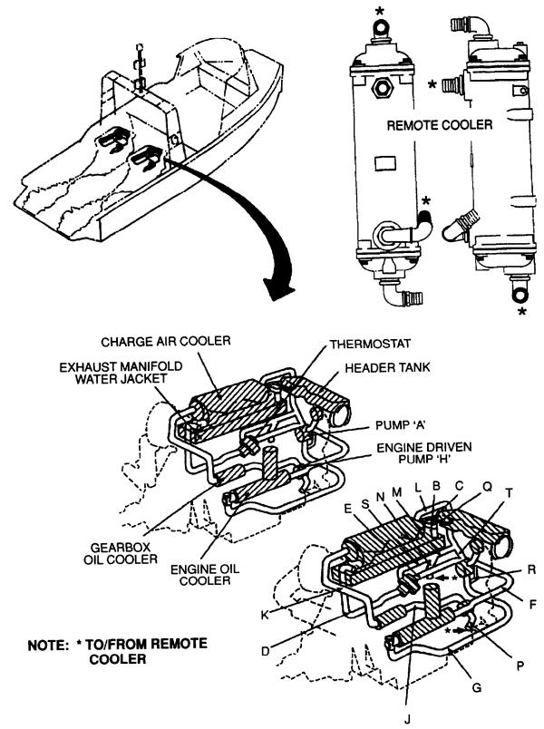
MK 1 FRESH WATER ENGINE COOLING SYSTEM
