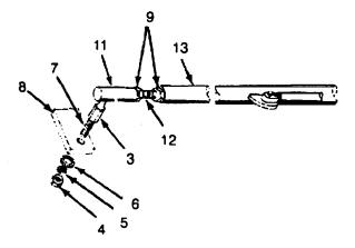
5. Pull linkage pin (7) out of hole in inner steering arm (8).
