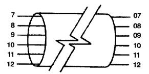
2. If continuity test fails, replace wiring harness with a serviceable wiring harness.
