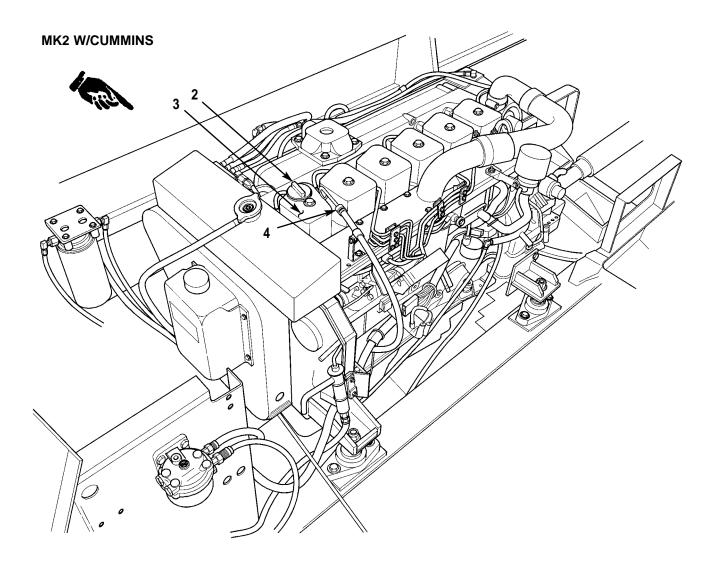
2. Using sump pump (1), pump used oil into five gallon container and discard.
