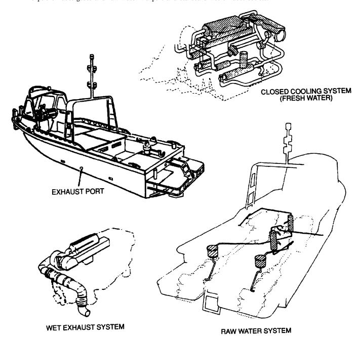
b. MK2. Each MK2 engine uses two closed cooling systems which share a common reservoir. The MK2 uses a wet exhaust system similar to the MK1. The hydrojet forces raw water into the exhaust system and out the exhaust port on the side of the boat.
